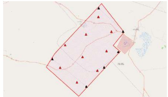
Illustration of location of GCP and control surfaces with given flight lines
